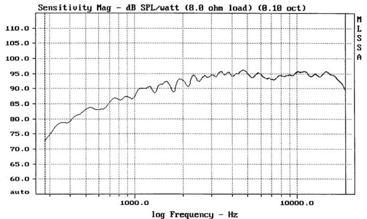
Driver is mounted rigidly in free air with no baffle or enclosure. Input signal is a stepped sinusoidal at 1VRMS. Impedance is measured using constant-voltage method. No smoothing was applied.
